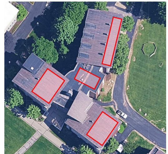
Solar array simulated rooftop location. Areas on the wings have a curved roof, while the center location is a flat roof.
