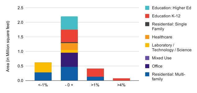
Percent Change in Construction Cost due to Net Zero in MA
